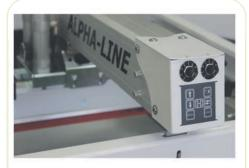
Touch-command in each printing head for start/stop/lift up-down/squeegee-drive for test print half-start/return
